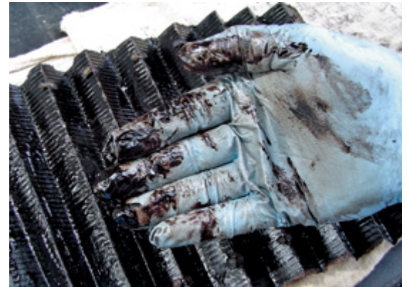
Sludge on an opened filter
